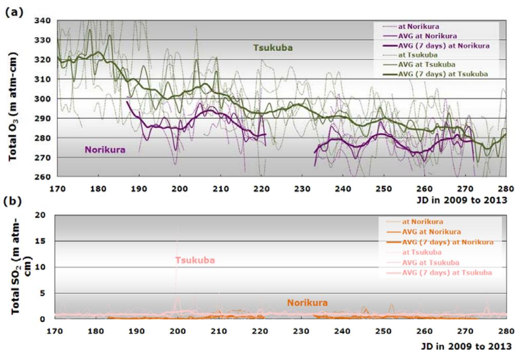
Fig. 5 Trends of daily mean of total O<sub>3</sub> and total SO<sub>2</sub> with Brewer Spectrophotometers at Norikura and Tsukuba from 2009 to 2013. Upper figure (a) show the daily mean of ds O<sub>3</sub>, and lower figure (b) shows the daily mean of ds SO<sub>2</sub>, respectively. Heavy lines indicate the seven day -running means of the daily mean for five years.
