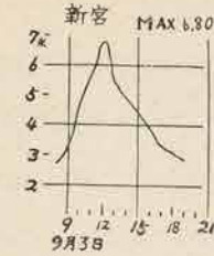
Fig. 5.2.18 Water-level of Dozan River
