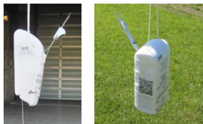
Photo 1 Model iMS (left) and 11G (right) GPS sondes.
